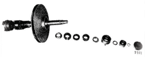
D. Outboard rotating element components removed, illustrating disassembly order.
