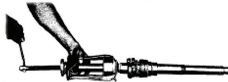
F. Impeller removed from outboard rotating element. G. Removing bearing from shaft using conventional puller.
