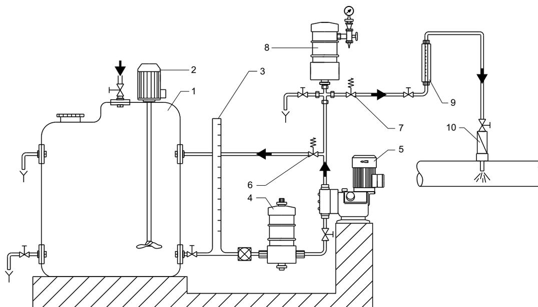
Fig. 46 Overview of a dosing system
