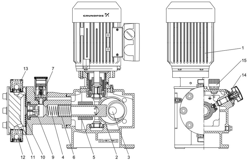
Fig. 19 Sectional drawing, DMH model 254
