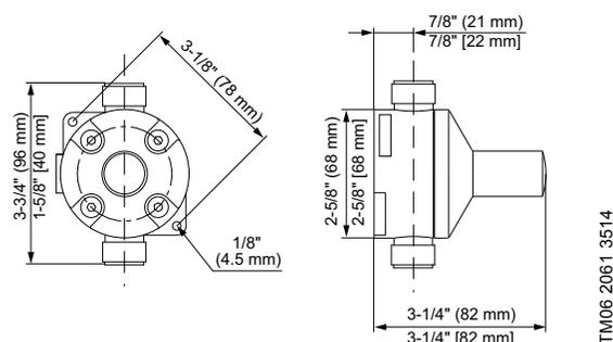
Fig. 44 Pressure loading valve. Dimensions in brackets apply to stainless-steel version.
