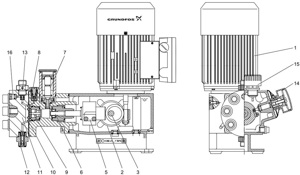
Fig. 22 Sectional drawing, DMH model 280
