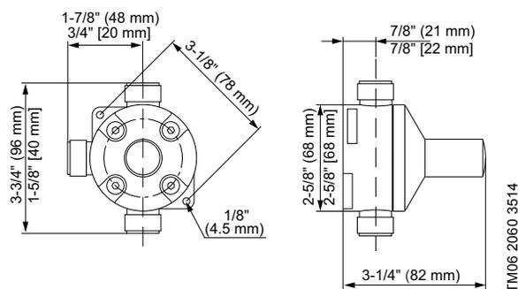
Fig. 43 Pressure relief valve. Dimensions in brackets apply to stainless-steel version
