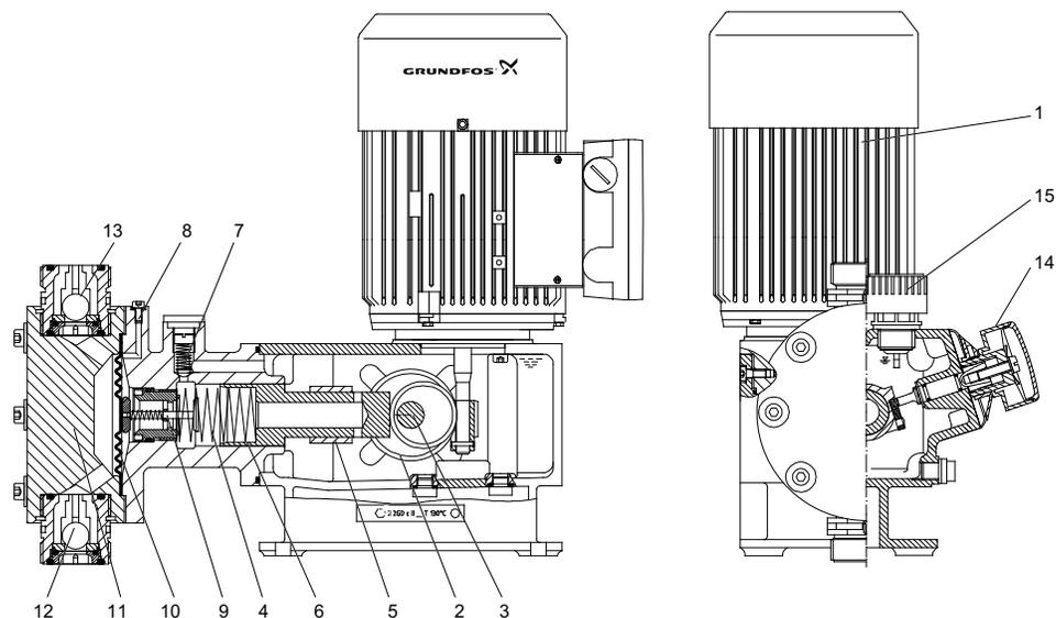
Fig. 18 Sectional drawing, DMH model 253
