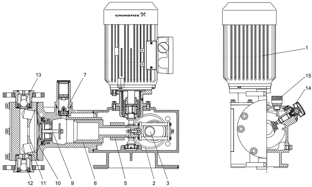
Fig. 21 Sectional drawing, DMH model 257
