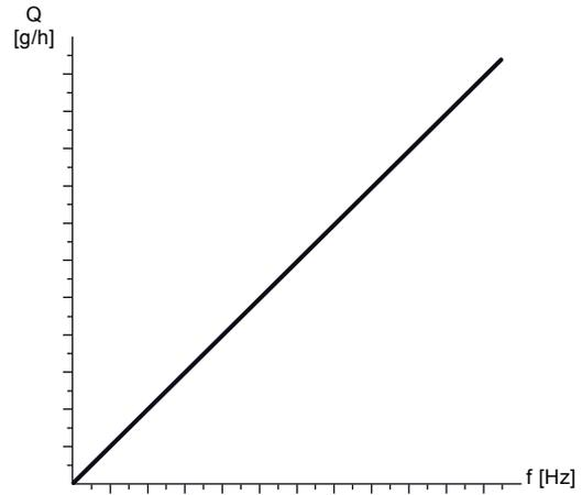
Fig. 6 Relation of motor frequency - capacity
