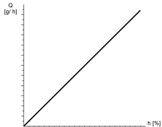
**Fig. 3** Relation of stroke length and capacity
