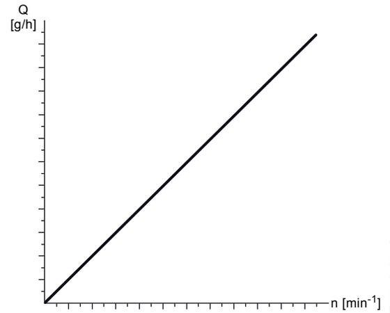
Fig. 8 Relation of stroke frequency - capacity
