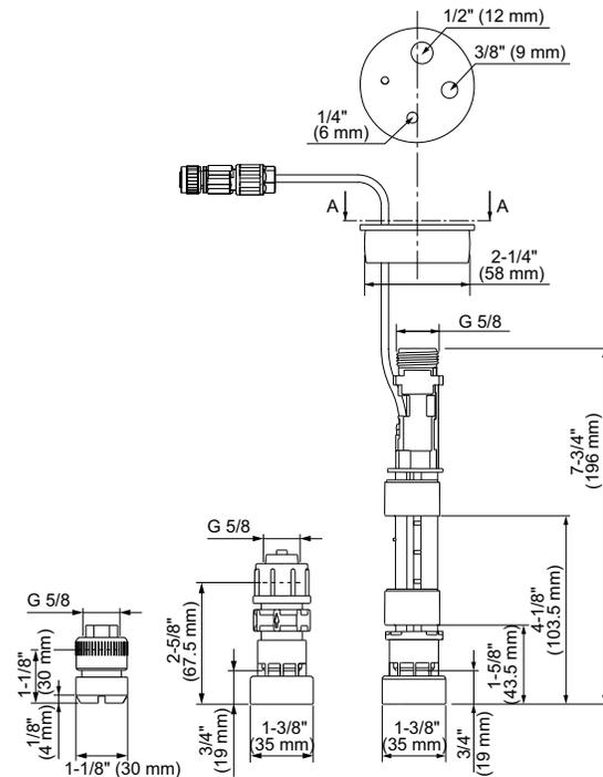
Fig. 32 Left: stainless-steel foot valve; center and right: PE or PVDF foot valve, dimensions
