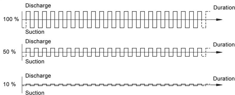
**Fig. 4** Relation of stroke length adjustment - capacity
