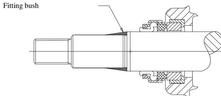
If the carbon ring is not fixed, it is important to check that it is fitted correctly, i.e. the chamfered/lapped side is to face the seat. The carbon ring can be held by a little grease. When using oil on the shaft, the bellows will settle and seat in about 15 minutes, and until then tightness should not be expected. After start, check by viewing the leak hole that there are no leaks.
