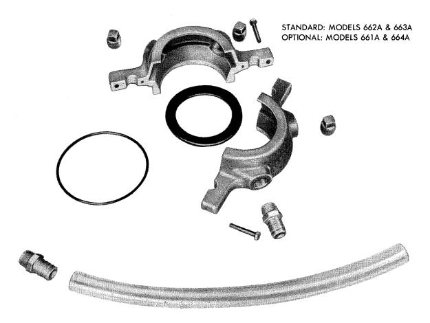
The leakage accumulator gland (sprayless, dripless packing gland) is designed and constructed to prevent the collection of packing leakage in the pump bracket of a vertical or horizontally mounted pump. The leakage accumulator gland has a volute shape with two symetrical halves. This gland encloses the water slinger preventing any spray from escaping and contaminating the area. The leakage is efficiently directed to a drain connection.
