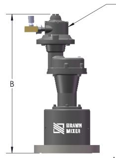
OPTIONAL AIR MOTOR INCLUDES MUFFLER AND NEEDLE VALVE. REFER TO TABLE FOR AIR SUPPLY REQUIREMENTS.
