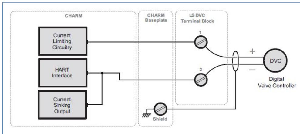
*Simplified Circuit and Connection Diagram for LS DO 24V DC ETA CHARM.*
