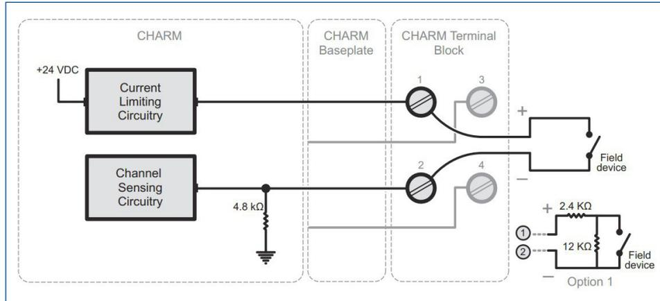
Simplified Circuit and Connection Diagram for LS DI 24V DC low-side sense CHARM.
