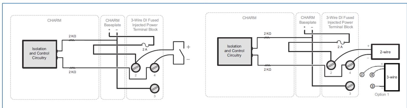
Simplified Circuit and Connection Diagrams for LS DI 24V DC Isolated CHARM with 3-wire DI Fused Injected Power Terminal Block.
