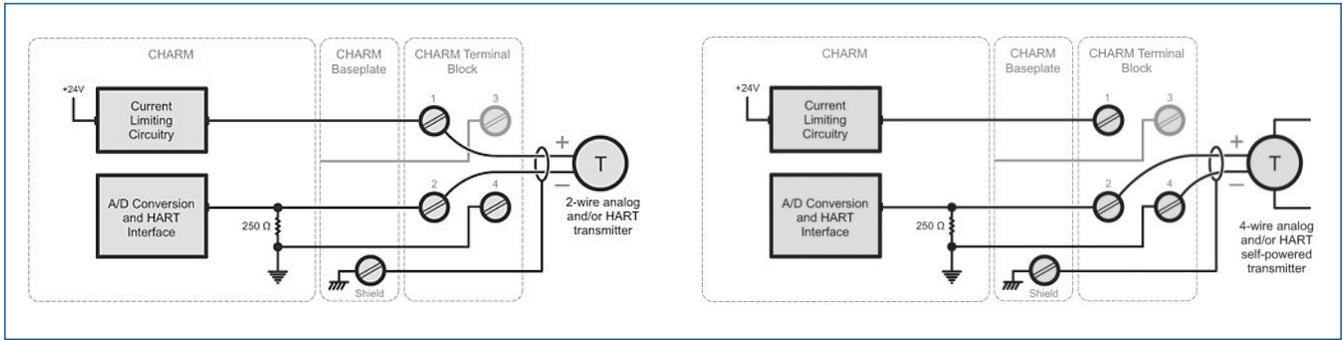
Simplified Circuit and Connection Diagrams for LS AI HART CHARM 0/ 4 to 20 mA Two Wire and Four Wire transmitters.
