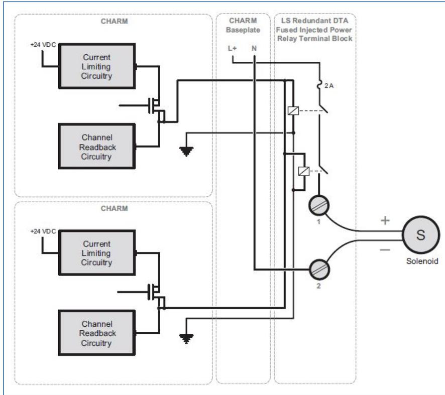
Simplified Circuit and Connection Diagram for LS DO 24V DC Redundant DTA CHARM with LS Redundant Terminal Block.
