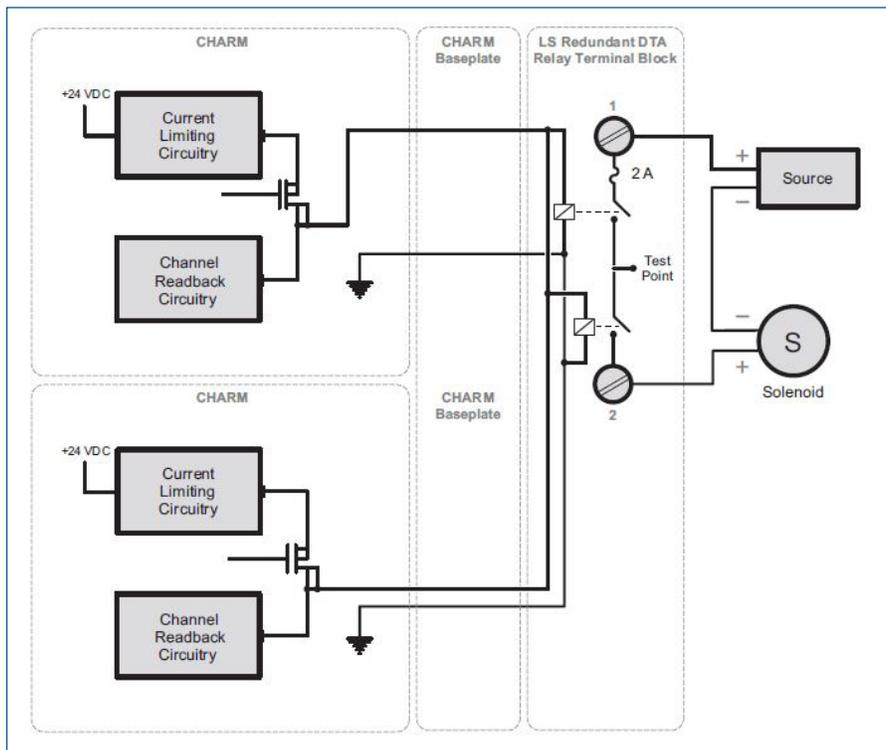
Simplified Circuit and Connection Diagram for LS DO 24V DC Redundant DTA CHARM with LS Redundant DTA Relay Terminal Block.
