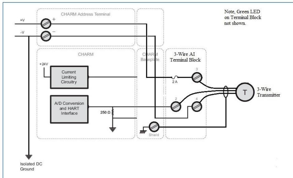
Simplified Circuit and Connection Diagrams for AI HART CHARM 0/ 4 to 20 mA with 3-wire AI Fused Injected Power Terminal Block.
