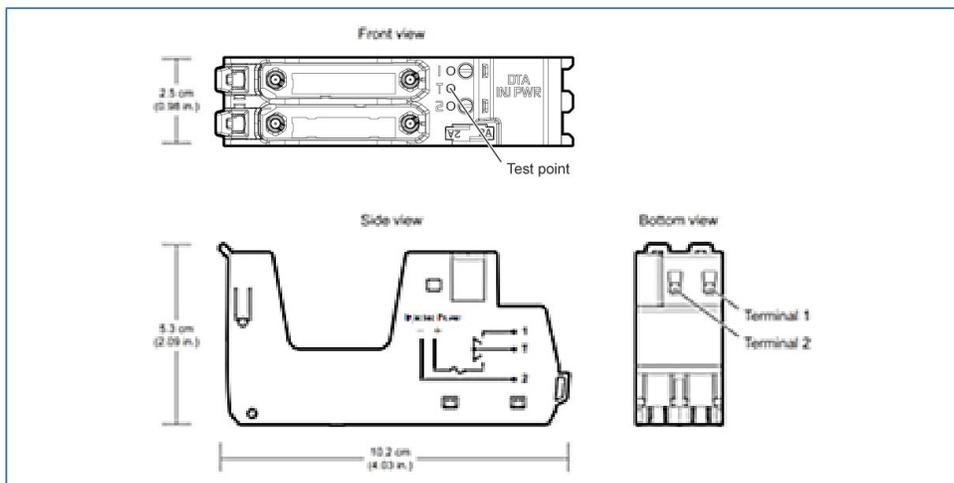
LS CHARM Redundant DTA Fused Injected Power Relay Terminal Block.
