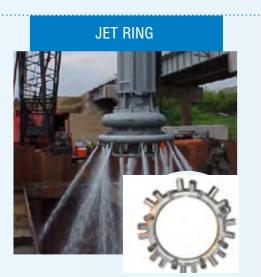
The jet ring **delivers high pressure water** through nozzles to loosen up compacted and heavy solids and thus fluidizing dense solids mixtures into the intake of the pump.
