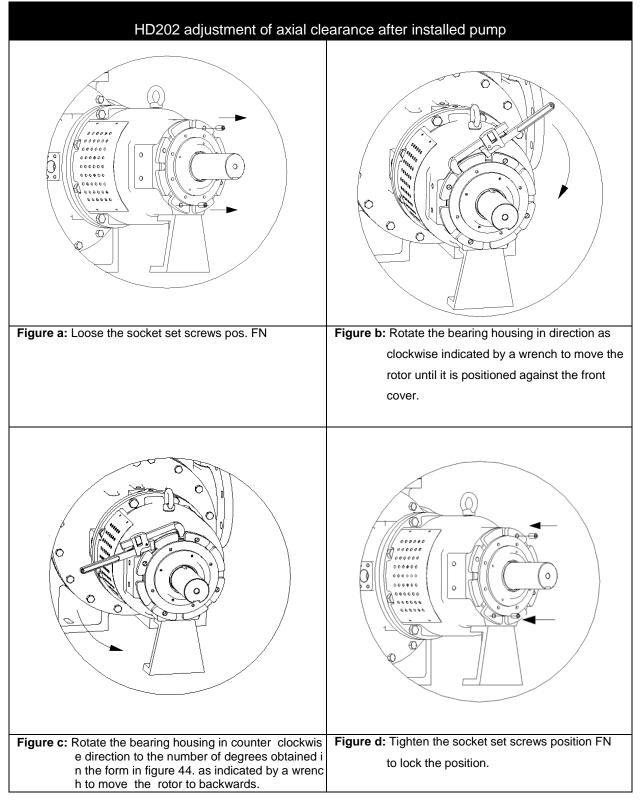
Figure 48:The procedure for setting the axial clearance on installed and non-installed HD202 pumps.
