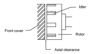
Figure 42:The axial clearance between the rotor/idler and the front cover.
