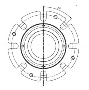
Figure 46:HD202 axial clearance adjustment - adjust the bearing housing(pos. CR) .
