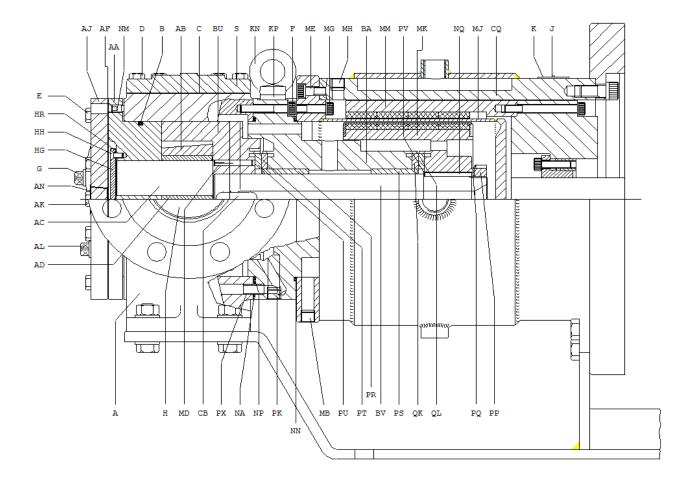
Bypass valve for HD,GP (CD,PD,ED)
