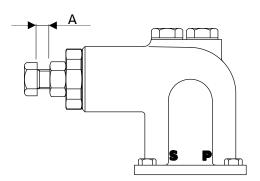
Figure 28:The setting value "A" for ROTAN valves.
