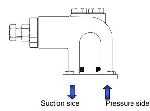
Figure 26:: Shows how S for suction side and P for pressure side are indicated on the valve.
