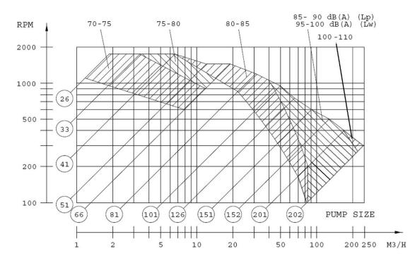
Figure 33:The maximum A-weighted sound pressure level in dB(A)(Lp) for the various pump sizes in relation to the pumps' flow. The range above 85 dB(A) is also expressed as sound power level (Lw).
