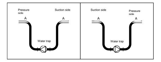
Figure 18: Shows a simplified sketch of a pump (the circle) fitted in a water trap.
