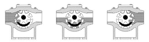
Figure 2:Shows the liquid flow through the ROTAN pump – seen from the front end.
