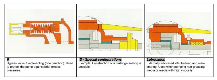
Figure 8:The codes of the various pump versions together with an explanation of what they mean.
