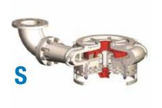
The **S Wet End** is a fantastic semi-open, high efficiency, solids handling pump. This wet end is capable of handling Class 1, 2, & some Class 3 slurries. It boasts a special elliptical cut-water design which maximizes efficiencies and reduces wear.
