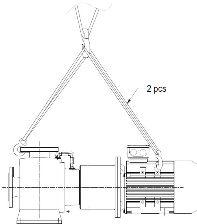
The lifting straps must not bear against sharp edges and corners.
