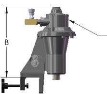
OPTIONAL AIR MOTOR INCLUDES MUFFLER AND NEEDLE VALVE. REFER TO TABLE FOR AIR SUPPLY REQUIREMENTS.
