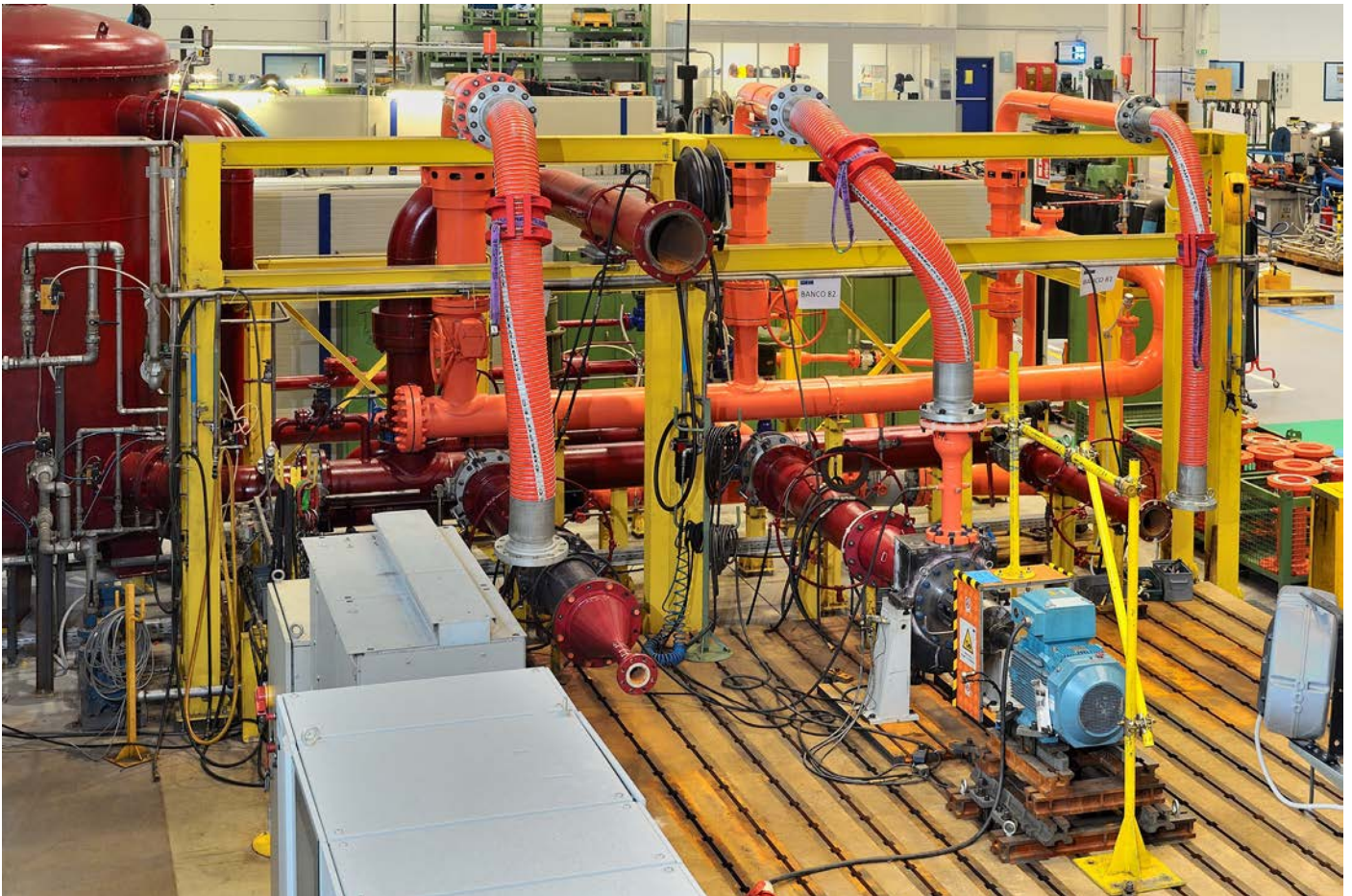
Gabbioneta Test Room – R pumps benches
