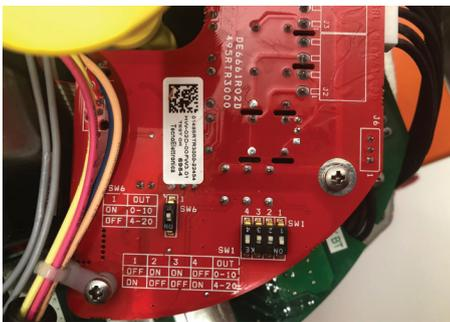
**OM1: input/output module** offers analog positioning control and position feedback, 4 additional SPST output contacts (configurable) independently settable at 10 points along the stroke, optional Bluetooth interface, information about loss of input signal and Bluetooth failure, and a local selector position alarm (with OM3 installed).
