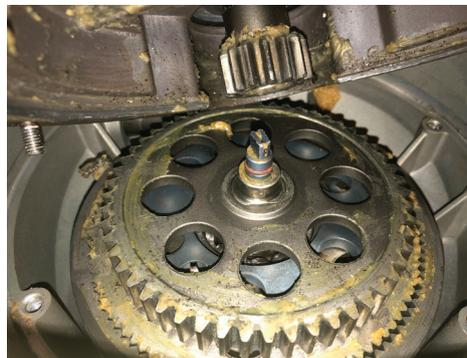
**Robust materials** are selected for loaded parts; for example, sintered alloy epicyclic gearing and cast-iron output drives.
