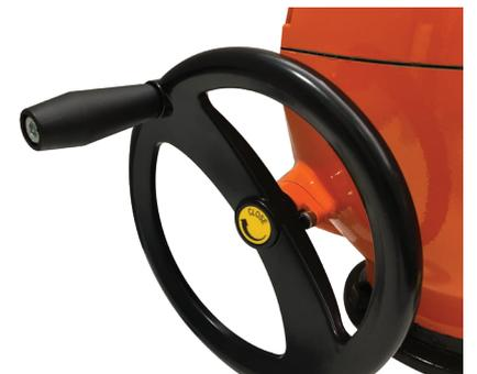
**Manual override** is always engaged, featuring a handwheel that does not rotate while the motor is in operation. This feature can be used when power to the actuator is lost.
