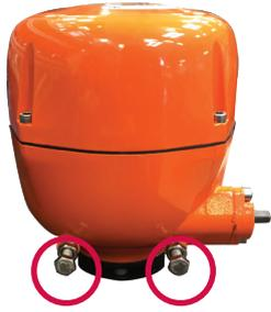
**Mechanical travel stops** at the base of the enclosure prevent over-travel during operation with the handwheel or motor, providing  $\pm 10^\circ$  of over/under travel in each direction (resulting in  $70^\circ$  minimum and  $110^\circ$  maximum angular stroke).
