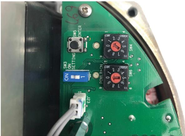
**Precise torque control** is configurable via user-friendly rotary switches located inside the control enclosure; bi-directional torque values of 50%, 75%, and 100% of nominal torque may be selected.
