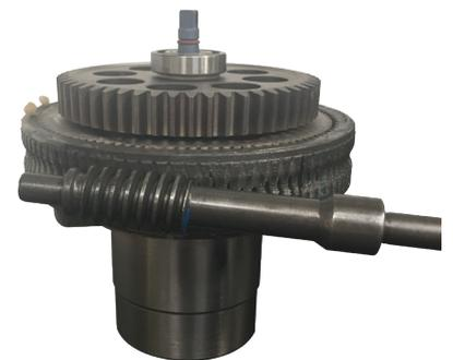
**Smooth gearing** is achieved with an all-metal, internally-located, greased, and self-locking epicyclic gearing system, which helps eliminate the need for motor brakes.
