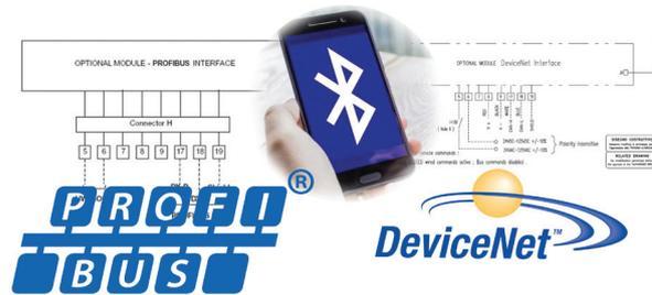
**Simple connection to a bus system** is possible with the optional OM9 (PROFIBUS DPV0/V1) and OM11 (DeviceNet) communication cards and setting all parameters via configuration software on a Bluetooth-enabled PC or PDA. Bluetooth is included as standard with the OM9 and OM11 cards.
