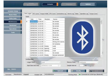
**Maintenance data for improved maintenance scheduling** (valve position, actuator speed, output torque, faults, and status) is directly accessible via optional Bluetooth connectivity.
