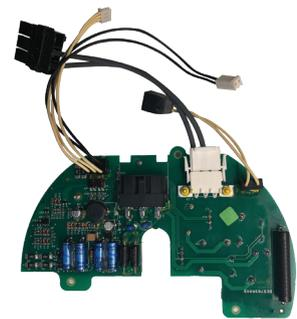
**OM13: 3-wire connection module** allows 120/240 VAC single-phase, 3-wire control for open/closed operations without an additional power supply.
