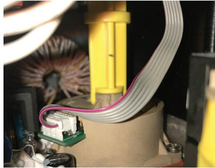
**Absolute position sensor** covers  $110^\circ$  of rotation, with travel endpoints set by the rotary switch (standard) or set non-intrusively (via optional Bluetooth).
