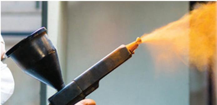
**Electrostatic powder coating** provides protection from the elements and is rated to 1,000 hrs minimum against salt spray and 100% humidity.
