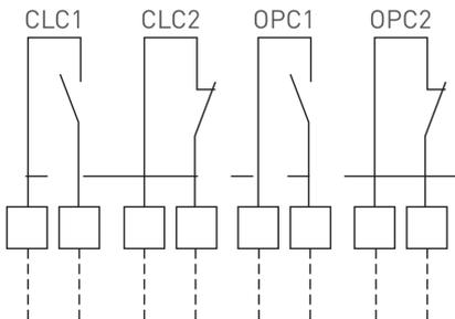
**Four latched-type output contacts** are available for remote indication of fully open or closed status. Output contacts for monitoring and blinker/local selector indication are also available.
