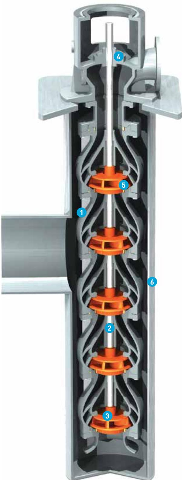
1. Accurately machined flanged bowl design promotes well contoured and smooth passageways. Bowl shaft supported by Rulon 123 bearings to provide excellent corrosion resistance.
