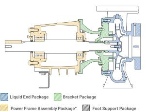
\*Power frame assembly package includes shaft & foot support package by default.
