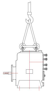
Screw lifting eyes into the pressure flange and mount lifting straps. The lifting straps must not bear against sharp edges and corners.
