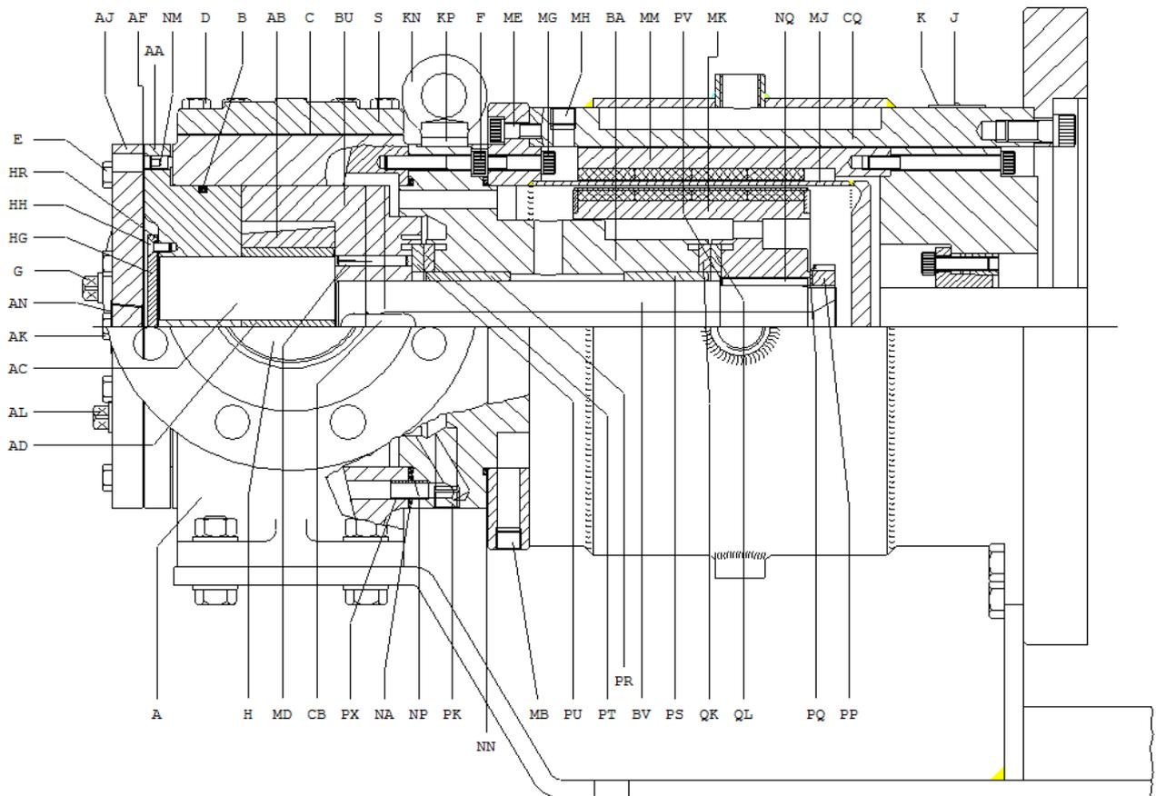
Bypass valve for HD,GP (CD,PD,ED)
