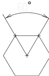
Figure 45: The size of the angle for a single surface on the hexagonal bolt head on the adjusting screws.
