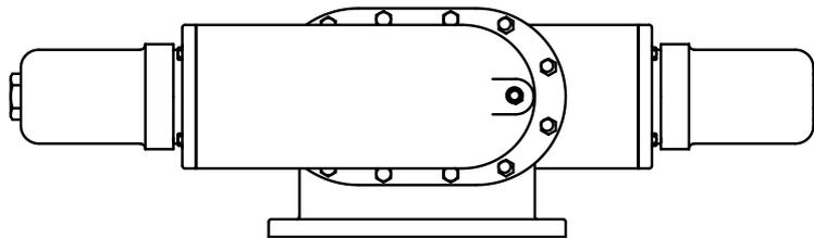
Figure 24: A double-action bypass valve.
