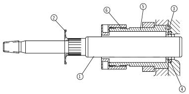
\*For both Stuffing Box and Gland use the following: Nickel Aluminum Bronze: xxxx-xxxx-01A. 316 Stainless Steel: xxxx-xxxx-03A. 2205 Duplex Stainless Steel: xxxx-xxxx-04A.
