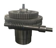
Smooth gearing is achieved with an all-metal, internally-located, greased, and self-locking epicyclical gearing system, which helps eliminate the need for motor brakes.
