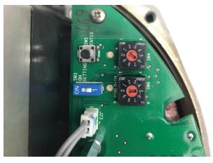
**Precise torque control** is configurable via user-friendly rotary switches located inside the control enclosure; bi-directional torque values of 50%, 75%, and 100% of nominal torque may be selected.
