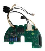
OM13: 3-wire connection module allows 120/240 VAC single-phase, 3-wire control for open/closed operations without an additional power supply.
