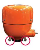
Mechanical travel stops at the base of the enclosure prevent over-travel during operation with the handwheel or motor, providing ±10° of over/under travel in each direction (resulting in 70° minimum and 110° maximum angular stroke).
