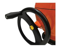
Manual override is always engaged, featuring a handwheel that does not rotate while the motor is in operation. This feature can be used when power to the actuator is lost.
