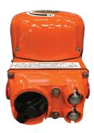
OM3: local interface module offers local/ remote selection, open/closed push-buttons, and two LEDs for local indication (note: OM3 is available in weather-proof version only).
