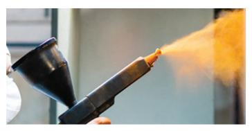
**Electrostatic powder coating** provides protection from the elements and is rated to 1,000 hrs minimum against salt spray and 100% humidity.
