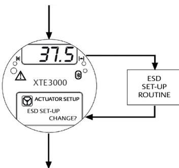
**Emergency Shut Down (ESD)** signal can override any existing control and move the valve to a predetermined position of your choice (actuator must be connected to main power supply for ESD to function).
