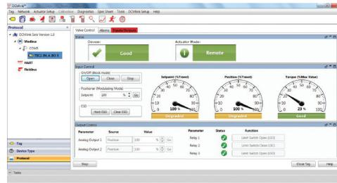
**Maintenance data** viewable on DCMLink includes full internal data-logger records, operating data, alarms, valve torque curves, and provides important information on the performance and operating condition of valves and systems.
