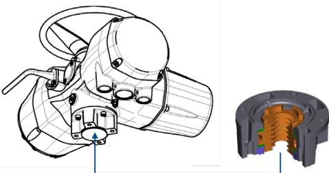
**Detachable coupling** (thrust base) can be removed from the actuator and mounted to the valve independently, which means that the whole actuator does not need to be spun on to the valve during installation.
