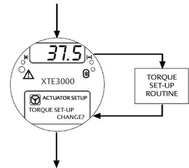
**Torque and valve position** can have their endpoints customized as a function of valve position (anywhere from 0-100%) or set to specific torque values.
