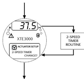
**2-speed timer** routine can extend valve operating time in the opening or closing direction.
