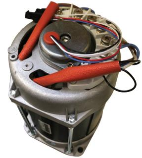
**Speed sensor** on the motor is equipped with a microprocessor to accurately record torque data. A thermostat also resides on top of the motor, which trips the motor if it over-heats (caused by the actuator being pushed beyond its rated torque).
