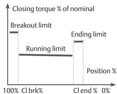
**Limit position** from 0% to 100% of the open position (0% = closed).
