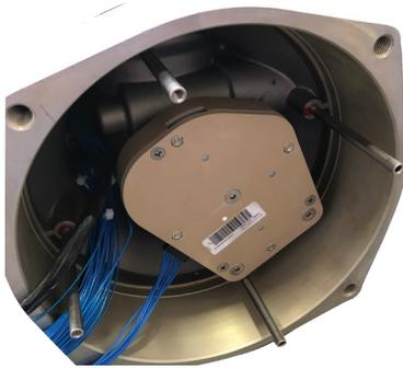
**Simple and robust** absolute position encoder sensor with high reliability and accuracy, which allows for position detection even when mains and back-up power are lost. Position accuracy is within 0.1% of true position, and position is recordable up to 8,580 full rotary cycles of the actuator's output shaft.
