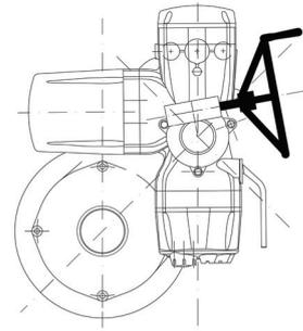
**Handwheel reducer** (a side-mounted 10:1 bevel gear) enables easier and smoother manual operation by reducing the load required to turn the handwheel.
