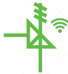
Pressure or Safety Relief Valve
